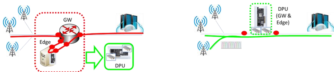
Figure A-18 - Today's reference scenario supporting edge computing through separated networking and computing resources (left); Edge computing node equipped with SmartNIC/DPU enhanced with coherent pluggable providing both networking and computing resources in a single platform (right).
