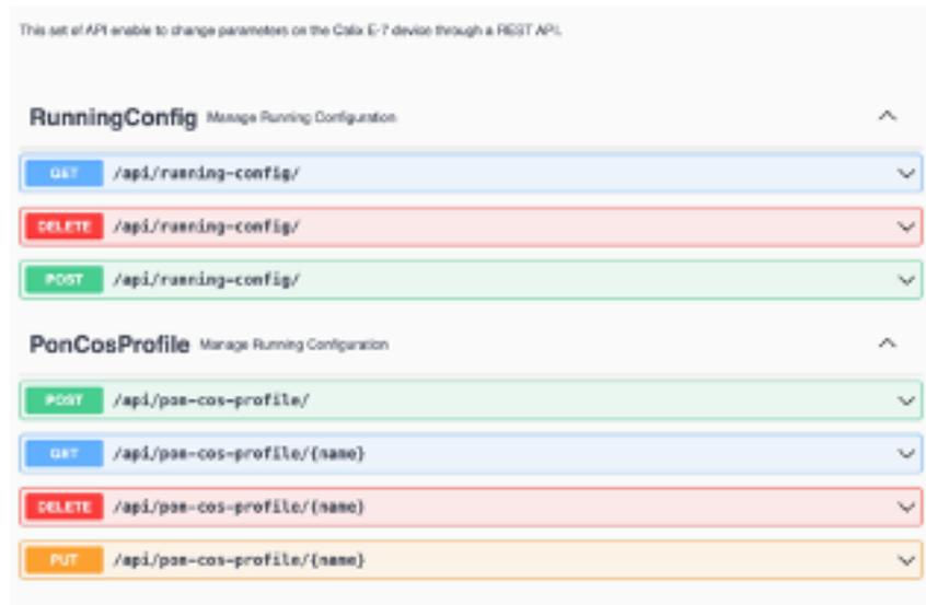
Figure 5.4: Optical Access Controller REST-APIs.
